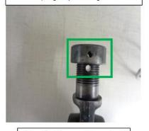
Step 3b- Shows alignment of the pin holes in nut and hook shank.
