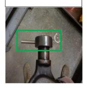
Step 5- Fully set the pin flush (could require some force with hammer) with one side of the nut, pin will not be flush with both sides of the nut.
